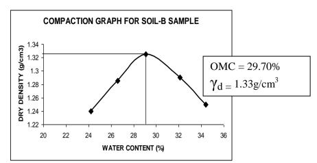
Fig 12: Variation of Dry density with different water contents for soil sample (B)
