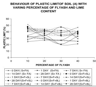
Fig 8: Behavior of plastic limit (%) of soil (A) with varying percentages of flyash and lime content
