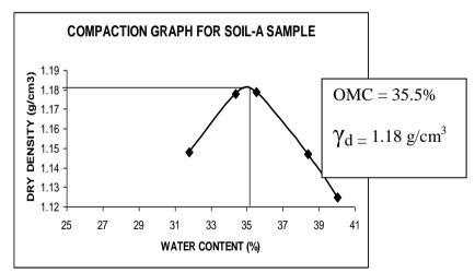
Fig 11: Variation of Dry density with different water contents for soil sample (A)
