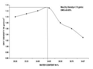
Fig 13: Variation of Dry density with different water contents of Flyash
