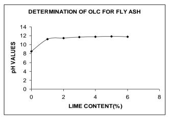
Fig 6: optimum lime content for fly ash by ph values
