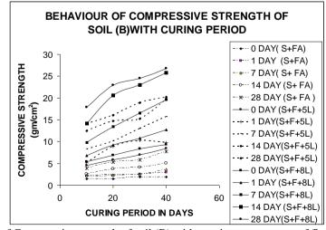
Fig 18: Behaviour of Compressive strength of soil (B) with varying percentages of flyash and lime content
