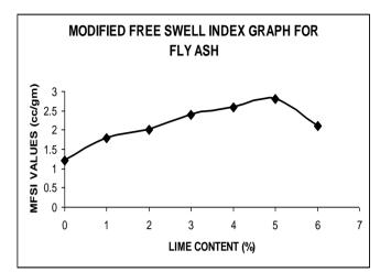
Fig 5: Variation of modified free swell index values with different lime content for flyash
