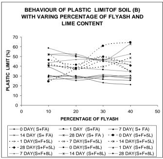
Fig 10: Behaviour of plastic limit (%) of soil (B) with varying percentages of flyash and lime content
