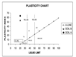
fig.2: Variation of plasticity index with the liquid limit of soil A, soil B.
