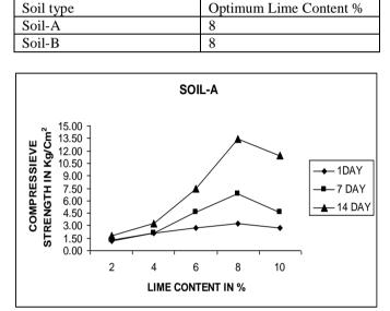
TABLE.1.3: Optimum lime content of soil A, soil B
